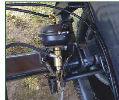
STR-305 Dual air and hydraulic brake system.
