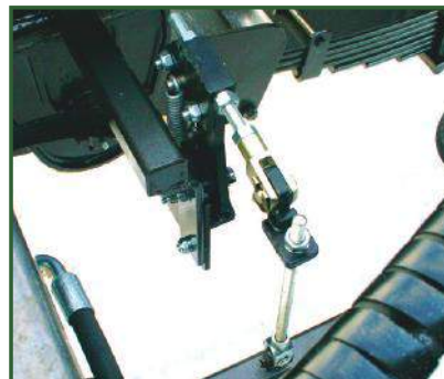
STR-302 Load sensing for hydraulic brakes.
