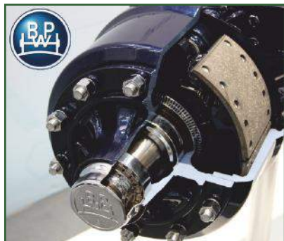
STR-211 BPW auto-centring free steering rear axle, 420x180 brake axles, 120x120mm square beam.
