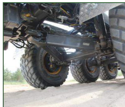
STR-410 Hydraulic suspension for optimal axle travel. Developed for heavier applications, both on and off-road.
