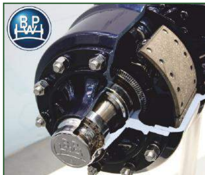
STR-211 BPW auto-centring free steering front axle, 420x180 brake axles, 120x120mm square beam.
