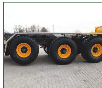
STR-411 Front lift axle - only available with air or hydraulic suspensions.
