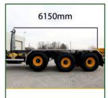
Length from tele-tower to rear roller – **6150mm.**
