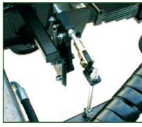
**STR-302** Load sensing for hydraulic brakes.
