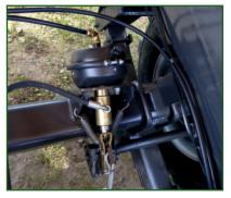
**STR-305**Dual air and hydraulic brake system.
