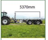
Length from tele-tower to rear roller – **5370mm.**
