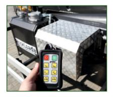
**STR-704** Independent hydraulic system with PTO, 130 l/min pump. Distributor operated by remote control.
