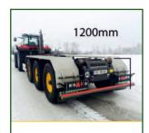
Roller height – **1200mm.**• Lowest roller height for a large-scale 25 tonne hook-lift trailer
