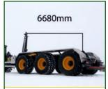
Length from tele-tower to rear roller – **6680mm.**
