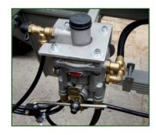
**STR-304**Load Sensing Valve (LSV) for air brakes.
