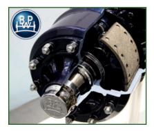
**STR-210**BPW high speed commercial axle, 410x180 brake axles, 120x120mm square beam, 10 stud.
