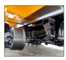
**STR-407**32t parabolic sprung suspension,
