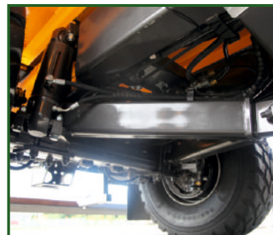
STR-410 Hydraulic suspension for optimal axle travel.
