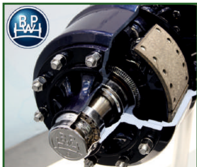
BPW commercial 410x120mm brake axles, 150x150mm square beam.
