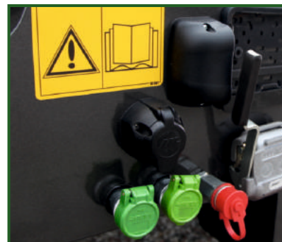
STR-1039 Rear mounted light connection 7- pin socket.
