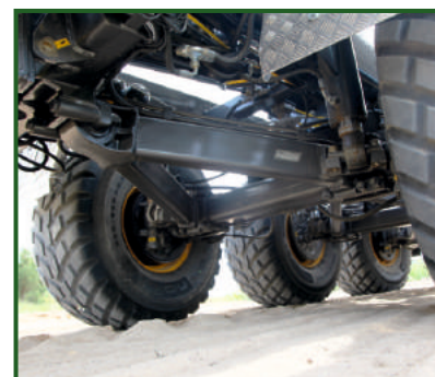
STR-410 Hydraulic suspension for optimal axle travel.
