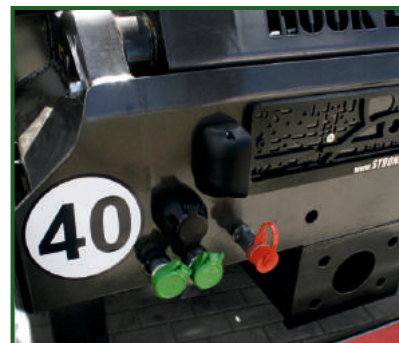
STR-1038 Rear mounted hydraulic brake connection.
