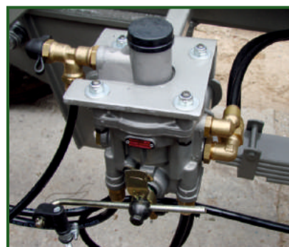
STR-304 Load Sensing Valve (LSV) for air brakes.
