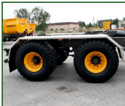
STR-406 24t parabolic sprung suspension, 1810mm distance between axles.
