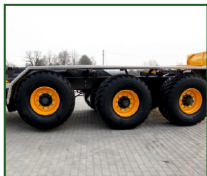
STR-411 Front lift axle - Only with air or hydraulic suspensions.
