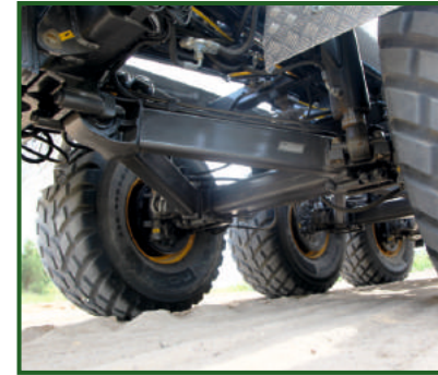
STR-410 Hydraulic suspension for optimal axle travel.
