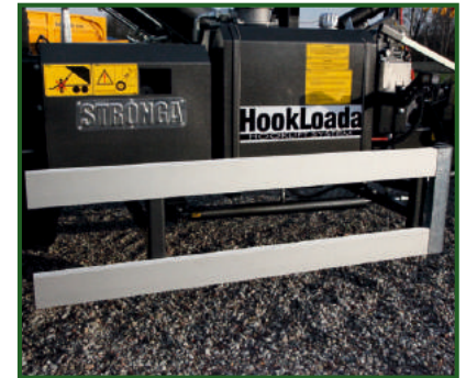
STR-1001 Aluminium side protection rails.
