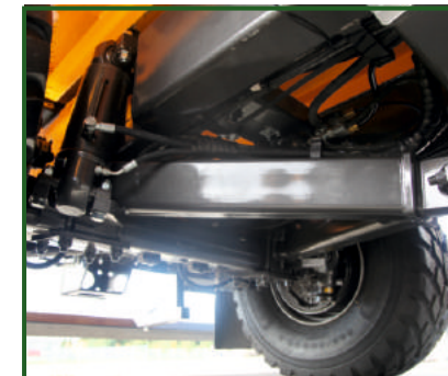
STR-410 Hydraulic suspension for optimal axle travel.
