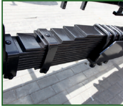
STR-501 Multi-position sprung drawbar for high comfort at speed.
