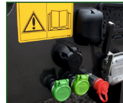
STR-1039 Rear mounted light connection 7-pin socket.
