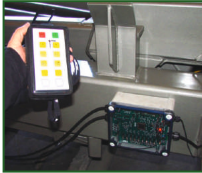
Independent hydraulic system with PTO. Distributor operated by remote control.
