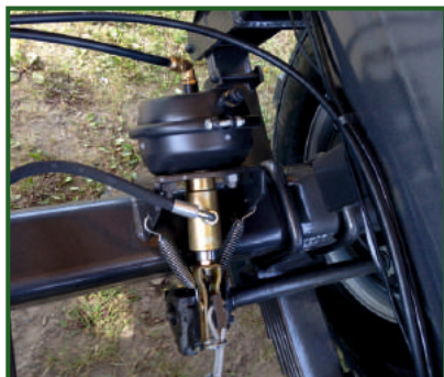
STR-305 Dual air and hydraulic brake system.
