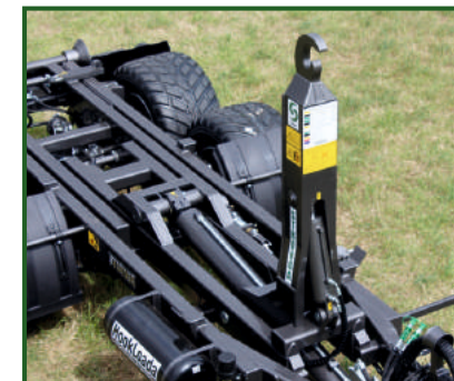
Tiltable hook tower with hydraulic cylinder.
