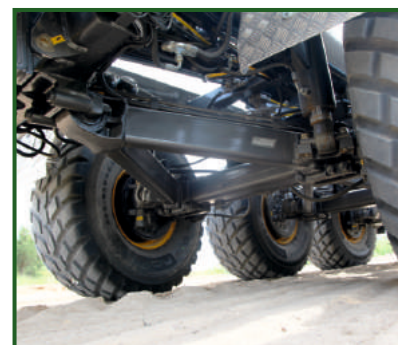
STR-410 Hydraulic suspension for optimal axle travel.
