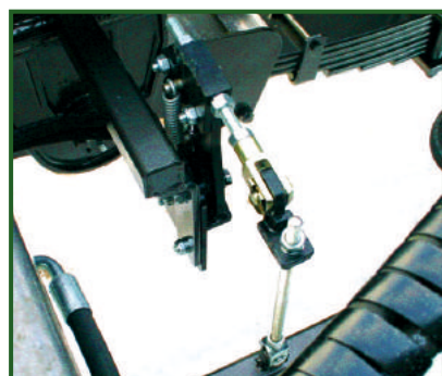
STR-302 Load sensing for hydraulic brakes.
