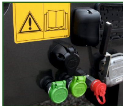
STR-1039 Rear mounted light connection 7-pin socket.
