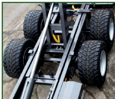
560/45 R22,5 152 D Nokian Country King TL. Load rating per tyre: 4840kg @ 40km/h 3550kg @ 65km/h
