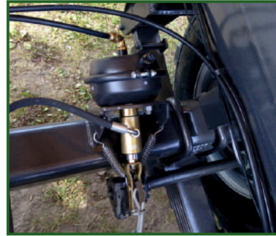
STR-305 Dual air and hydraulic brake system.
