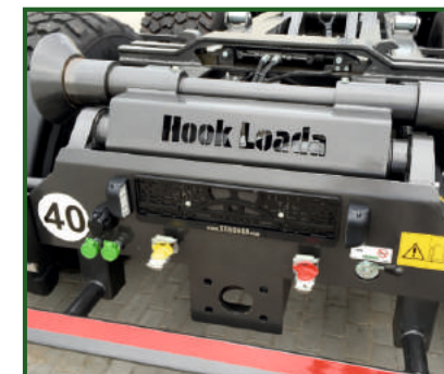
STR-723 Auxiliary hydraulic connections with electrical changeover valve at the rear of the trailer.
