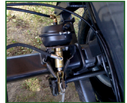
STR-305 Dual air and hydraulic brake system.
