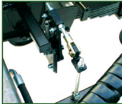
STR-302 Load sensing for hydraulic brakes.
