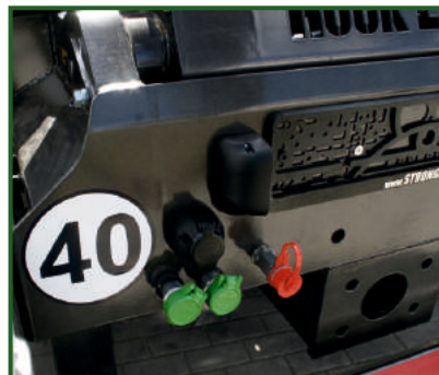
STR-1038 Rear mounted hydraulic brake connection.
