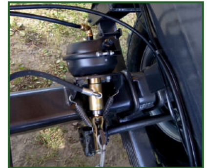
STR-305 Dual air and hydraulic brake system.
