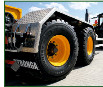
STR-900 Full length ultra-light aluminium mudguards.
