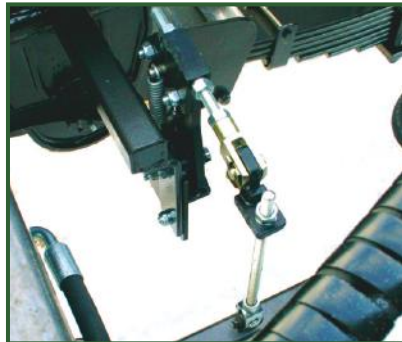
STR-302 Load sensing for hydraulic brakes.
