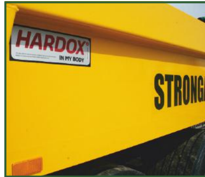
HARDOX 450 steel. 6mm floor. 4mm sides.
