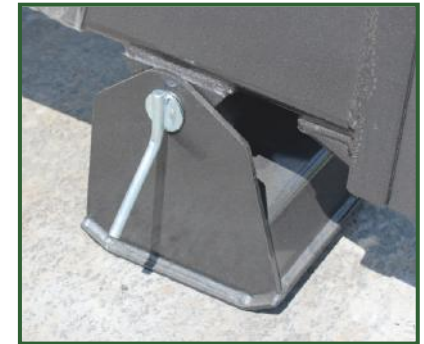
Suspended drawbar shoe with stowage point.
