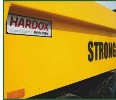
HARDOX 450 steel. 10mm floor. 8mm sides.
