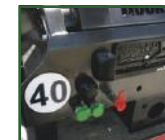
STR-1038 Rear mounted hydraulic brake connection.
