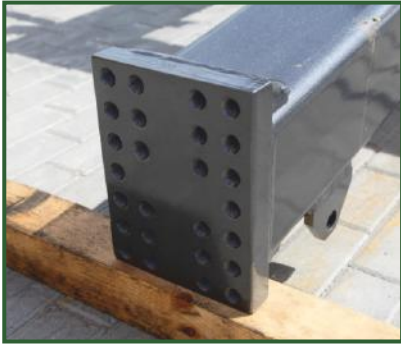
3 position plate for bolting towing eyelet.
