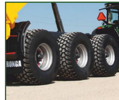
445/65 R22,5 radial tyres. Load rating per tyre: 7000 kg @ 105 km/h
