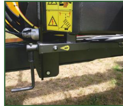
Cable-type hand brake.
