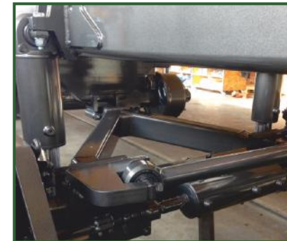
STR-410 Hydraulic suspension for optimum axle travel.
