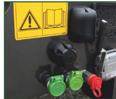
STR-1039 Rear mounted light connection 7-pin socket.
