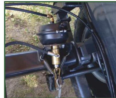
STR-305 Dual air and hydraulic brake system.
