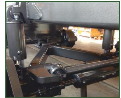
STR-410 Hydraulic suspension for optimum axle travel.
