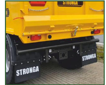
STR-1005 Multi-position removable round bumper at the rear of the trailer.
