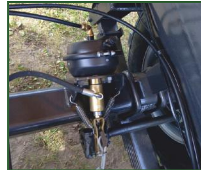
STR-305 Dual air and hydraulic brake system.
