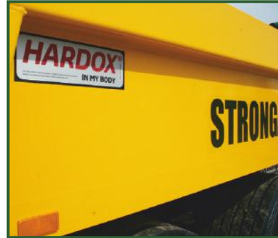
HARDOX 450 steel. 10mm floor. 8mm sides.
