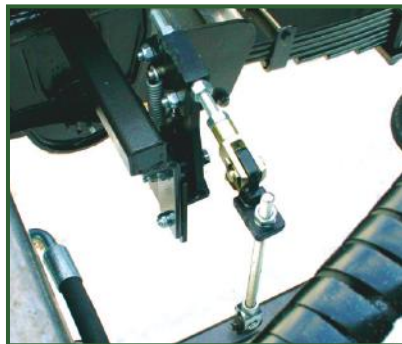
STR-302 Load sensing for hydraulic brakes.
