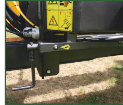
Cable-type hand brake.
