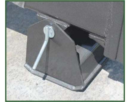
Suspended drawbar shoe with stowage point.
