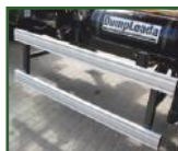
STR-1001 Aluminium, light-but-strong side protection rails.
