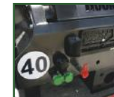
STR-1038 Rear mounted hydraulic brake connection.
