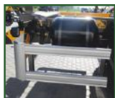
STR-1001 Aluminium, light-but-strong side protection rails.
