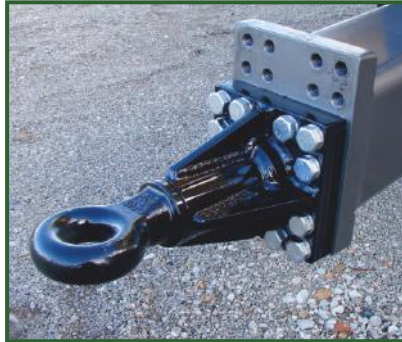
Swivel towing hitch. STR type. 50mm diameter eyelet.
