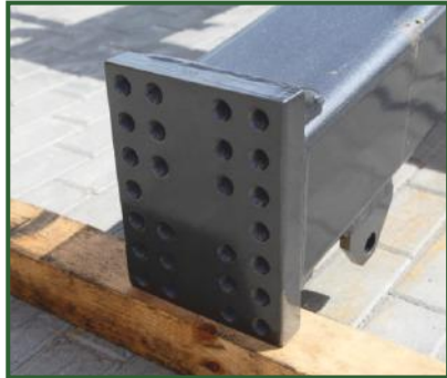
3 position plate for bolting towing eyelet.
