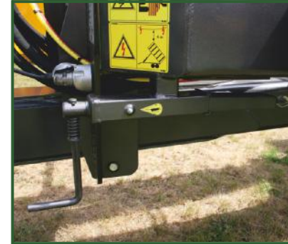
Cable-type hand brake.
