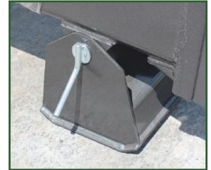
Suspended drawbar shoe with stowage point.
