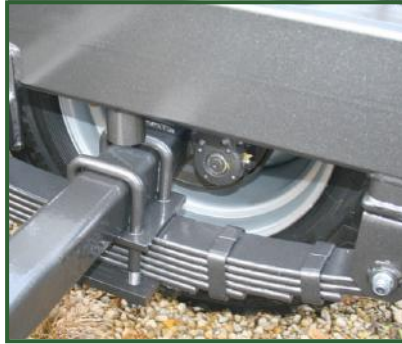
14t multileaf sprung suspension. 1480mm distance between axles.
