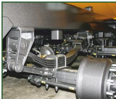
36t parabolic sprung suspension. 1525mm distance between axles. Springs under axles.
