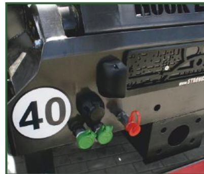
STR-1038 Rear mounted hydraulic brake connection.
