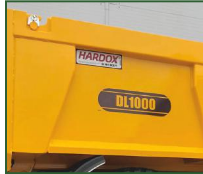
HARDOX 450 steel. 8mm floor. 6mm sides.
