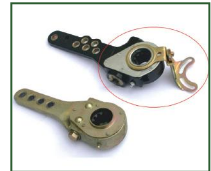
STR-307 Automatic slack adjusters.
