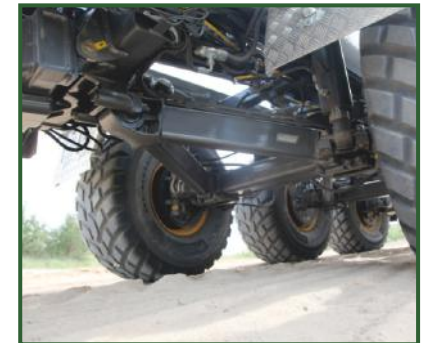
STR-410 Hydraulic suspension for optimum axle travel.
