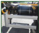
STR-1001 Aluminium, light-but-strong side protection rails.
