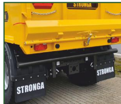
Multi-position removable round bumper at the rear of the trailer.
