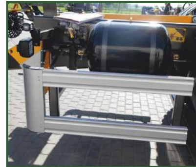
STR-1001 Aluminium, heavy-duty side protection rails.
