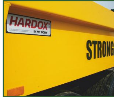
HARDOX 450 steel. 6mm floor. 4mm sides.
