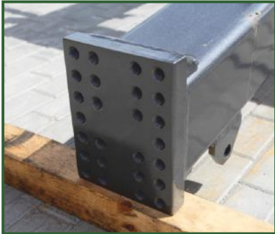
3 position plate for bolting towing eyelet.
