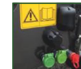
STR-1038 Rear mounted hydraulic brake connection.
