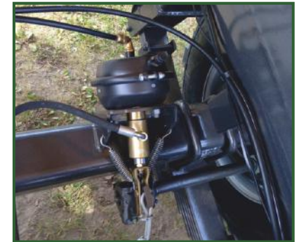
STR-305 Dual air and hydraulic brake system.
