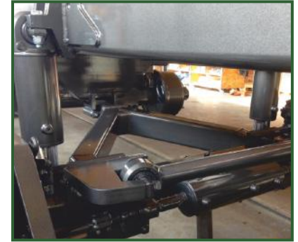
STR-410 Hydraulic suspension for optimum axle travel.
